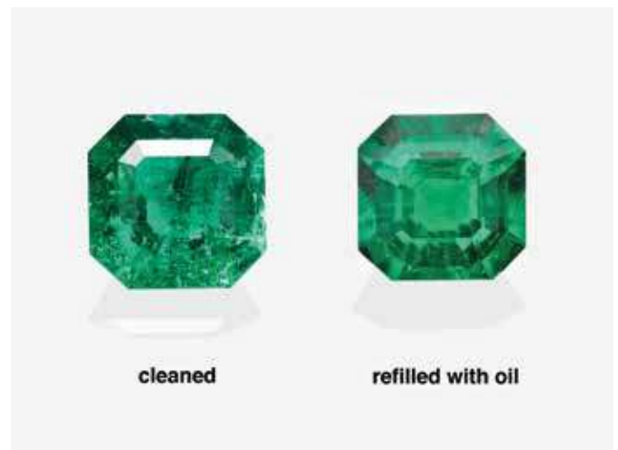
△ Figure 2: Colombian emerald which has been thoroughly cleaned (on the left) and which thus shows prominent fissures. After refilling these fissures with cedarwood oil, the apparent clarity of the same emerald (on the right) has distinctly improved. Both situations were analysed by SSEF and each time a report was issued, documenting the situation (first none, then moderate oil) at the time of each testing. Photo: L. Phan, SSEF
