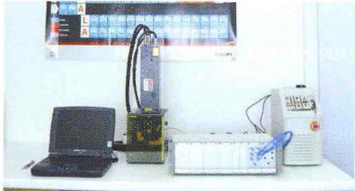
Figure 2 : An SSEF Gem LIBS system ready for application (Photo H.A. Hänni, SSEF)
