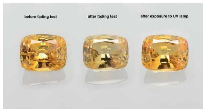
△ Figure 2: Yellow sapphire of >50 ct with unstable (reversible colour), seen before fading test (left), after fading test (middle), and after exposure to UV radiation (right). Photos: J. Kaysongkham, SSEF
