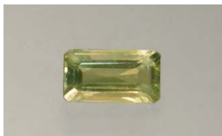
Figure 19: Light yellowish green or greenish yellow chrysoberyls such as this 2.44 ct gem (9.7×5.3 mm) typically contain – in addition to some Fe – small amounts of V and/or Cr (in this instance, microprobe analyses showed 0.77 wt.% Fe_2O_3 , 0.02 wt.% V_2O_3 , and 0.01 wt.% Cr_2O_3 ). Photo by K. Schmetzer.
