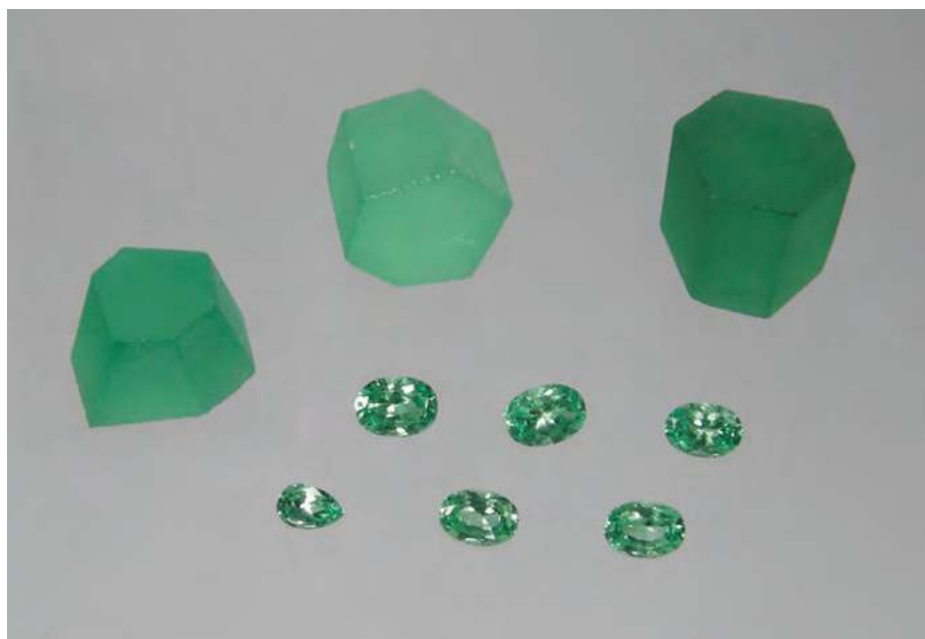
Figure 2: Rough and cut V-bearing synthetic chrysoberyl grown by Kyocera Corporation. The top-right piece weighs 10.5 g and measures 15.5×15.5×14.4 mm; the faceted samples weigh 0.49–1.33 ct. Photo by K. Schmetzer.
