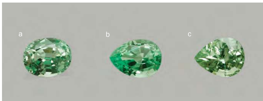
Figure 1: (a) Vanadium-bearing chrysoberyl was first discovered at Tunduru, Tanzania, which is the source of this 1.53 ct oval cut (7.8×6.2 mm). (b) Its synthetic counterpart was grown by Kyocera Corporation (here, 1.12 ct or 7.6×5.7 mm). (c) The Ilakaka area in Madagascar is also a source of V-bearing chrysoberyl; this sample weighs 2.09 ct and measures 9.1×7.2 mm. Composite photo by M. S. Krzemnicki (not to scale).
