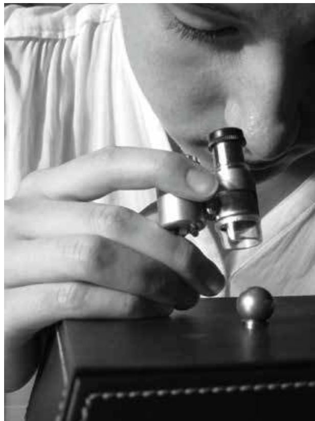
Figure 15: A pocket microscope can be used to read an HoP tag, and also to view the UV luminescence colour of the glue that is used to affix it. Photo by Jean-Pierre Le Pollès.
