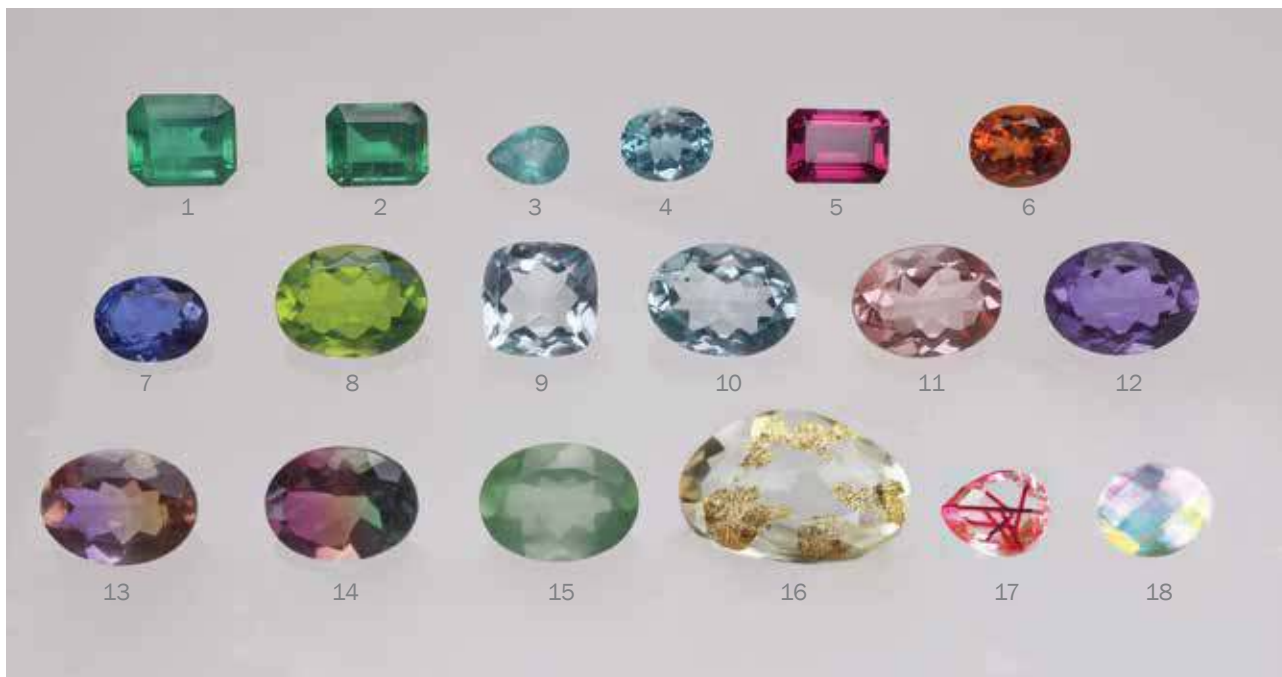
Figure 16: These doublets display various colours and optical effects. Samples 1–15 weigh 1.71–8.83 ct, and consist of colourless natural gemstone crowns and pavilions that are glued together with a coloured binder to create the illusion of popular gem varieties. The other samples weigh 2.29–13.79 ct, and display iridescence (no. 18) or contain pieces of foil in the cementing layer that produce different optical effects (nos. 16 and 17). Photo by H. A. Hänni.
