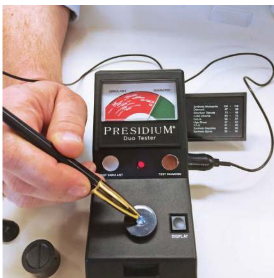
Fig. 2 Duotester in thermotester mode identifies blue diamond correctly as “diamond”
