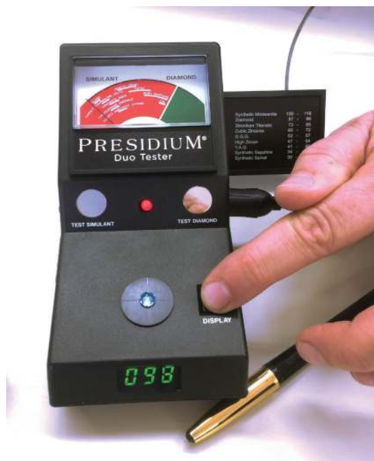
Fig. 3 Duotester in IR-reflectivity mode identifies blue diamond correctly as “diamond”
