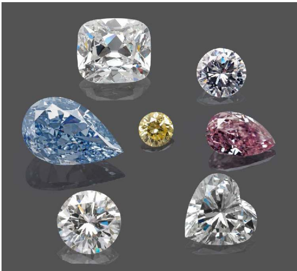
Figure 1: Seven colourless and fancy-colour diamonds (weighing up to 3.03 ct) of various natural or synthetic origins are shown here. The top-right and bottom-left round brilliants are HPHT- and CVD-grown, respectively, and the other diamonds are natural. The confident separation of natural and synthetic diamonds is critical to maintaining consumer confidence in the trade. Composite photo by Luc Phan, SSEF.
