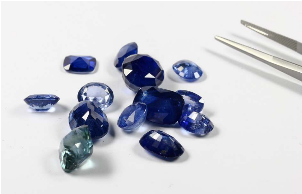
Figure 2: Sapphires heated with a new heating process, incorrectly named High Pressure-High Temperature (HPHT) heating in the trade.
