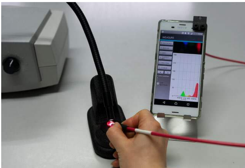
Figure 21: The set-up used for the experiments described in this report consisted of the GoSpectro device attached to a smartphone (Sony Xperia Z2), with the optional optical fibre and stand. A KL2 fibre-optic lamp (Schneider Gemmologie, Idar-Oberstein) was used as the light source. Photo by Q. Wang, German Gemmological Association.
