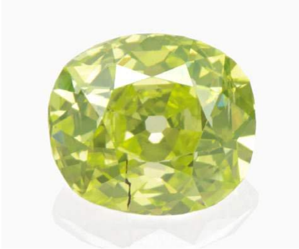
Figure 17: The 1.07 ct greenish yellow diamond described here was identified as having been artificially irradiated and annealed. Photo by Luc Phan, © SSEF.
