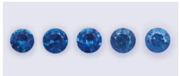
Figure 8: Five small calibrated spinels (from left to right: SPTan-2_1 to SPTan-2_5; each approximately 2 mm diameter; total weight 0.17 ct), reportedly cut from very dark rough from the same mining area near Lukande, were examined for this study. Photo by Alice Chalain, SSEF.
