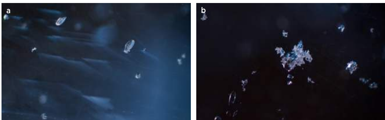
Figure 12: These inclusions in Lukande spinel consist of (a) dispersed apatite crystals and (b) a zircon cluster. Photomicrographs by M. S. Krzemnicki; magnified 50×.
