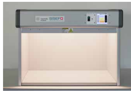
◁ The small light box operating with one of three available temperatures (here shown is 4500K). Photo: SSEF.
