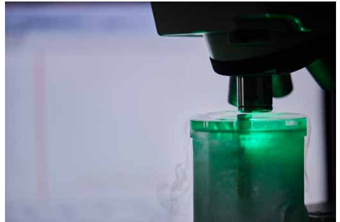
△ Low-temperature (-196°C) testing of diamonds in photoluminescence mode. Photo: SSEF.
