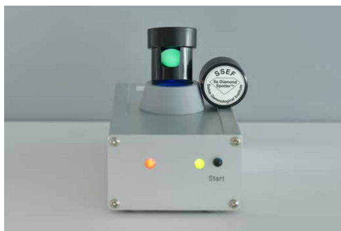
△ On the SSEF Instruments website you'll find a wide range of small gemmological instruments such as the SSEF Diamond Spotter which enables quick and easy identification of type IIa diamonds. Photo: SSEF.
