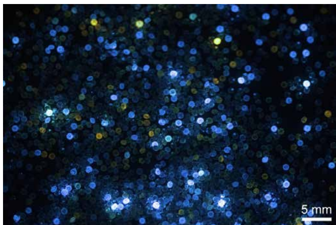
△ Figure 1: Fluorescence of the studied natural colourless diamonds observed under UV excitation (365 nm). Note that this fluorescence is typical of natural colourless diamonds. Figure: SSEF.
