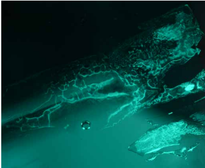
◁ Figure 1: Altered fissure filling substance (artificial resin) in an emerald fissure. Magnification 50x. Photo: M.S. Krzemnicki, SSEF.
