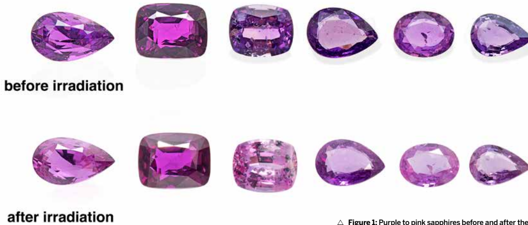
△ Figure 1: Purple to pink sapphires before and after the so-called 'hospital' irradiation treatment. As evident from the photo, the colour shift induced by the irradiation treatment varies from stone to stone from nearly no change to a rather distinct change. Photo: SSEF.
