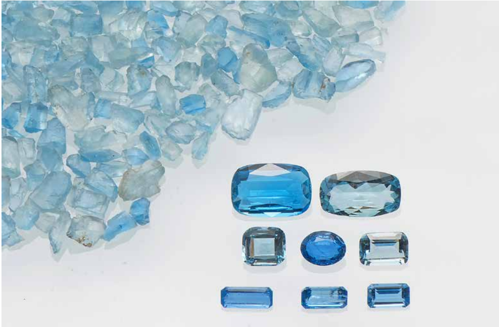
◁ Figure 1: Rough and faceted afghanite samples recently submitted to SSEF. The faceted afghanite samples range in weight from 0.2 ct to 4.2 ct, all are characterized by an attractive colour and exceptional clarity. Photo: J. Xaysongkham, SSEF.
