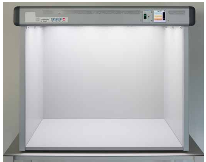
△ The large light box operating with one of three available temperatures (here shown is 6000K). Photo: SSEF.
